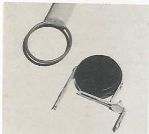
INDUCTANCE LOOP AND C PROBE ASSEMBLY
